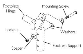
FIGURE 6.8 Installing Adjustable Angle Flip-up Footplate Hinge
